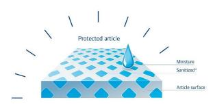
**GREENDEC® Sanitized®** consists of a **Polypropylene fabric cloth inner duct**, protected with the antimicrobial Sanitized® hygienic function to reduce bacteria growth, it reduces odor-causing bacteria, protecting the material permanently for peace of mind and more freshness.
