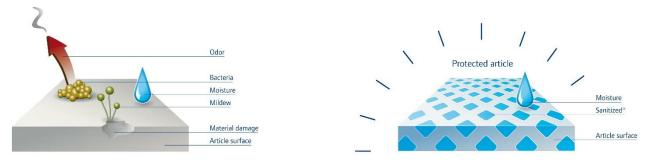
**GREENDEC®** Sanitized® consists of a Polypropylene fabric cloth inner duct, protected with the antimicrobial Sanitized® hygienic function to reduce bacteria growth, it reduces odor-causing bacteria, protecting the material permanently for peace of mind and more freshness.
